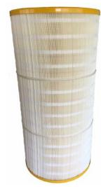
**FILTER UPGRADE:** The PTFE filter is a heavy duty synthetic spun bond filter with a high efficiency PTFE membrane covering the media. The PTFE membrane not only increases efficiency but also the dust releasing capabilities for superior cleaning. The PTFE media is washable, extremely rugged, and resistant to abrasives. This filter is designed for stainless welding and other weld processes requiring higher efficiency filtration.
